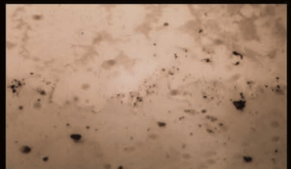
Cross cut sample etched in 50% HCL @ 800X
