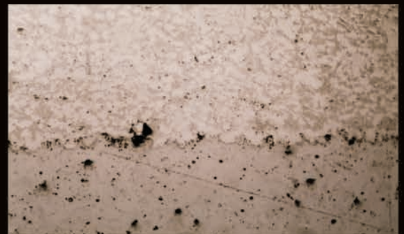
Cross cut sample etched in 50% HCL @ 200X
