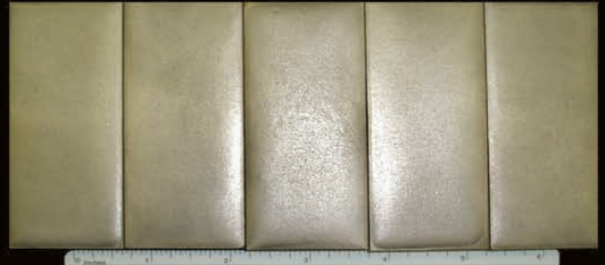
Finish surface using CermaClad process.
