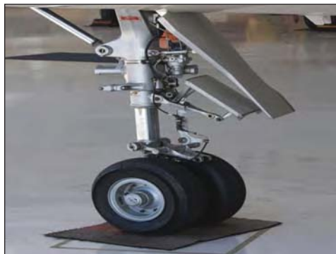
Fig. 1 — PComP coatings are a direct replacement for chromium plating currently used to protect landing gear from corrosion and wear.
