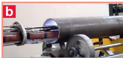
Fig. 1a) Operating principle (courtesy Vortek-Mattson industries) b) Setup for cladding inside a pipe
