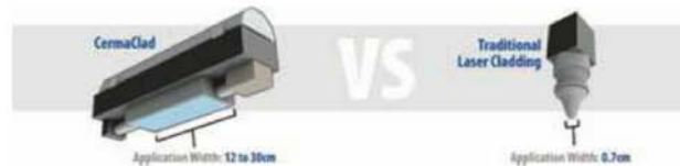
Figure 2: CermaClad arc lamp's 40 times wider application area compared to weld overlay coupled with rapid fusion, low heat affected zone, minimal dilution and porosity enables MesoCoat to produce clad pipes at rates up to 100 times faster than weld overlay.
