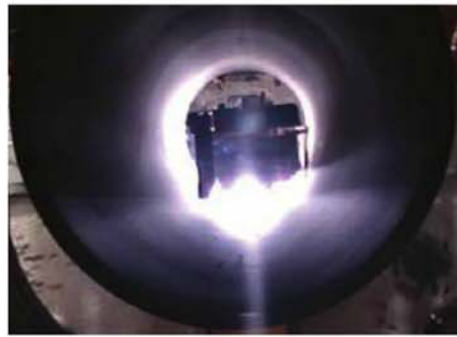
Figure 3: CermaClad high intensity arc lamp cladding the inside diameter of pipe with 3 mm thick Alloy 625
