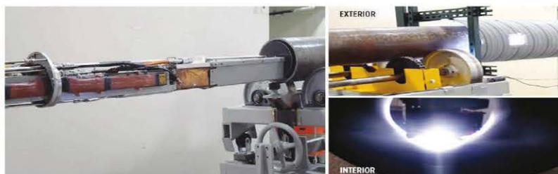
FIGURE 2: CERMACLAD HIGH INTENSITY ARC LAMP CLADDING THE INSIDE DIAMETER OF PIPE WITH 3 MM THICK ALLOY 625.
