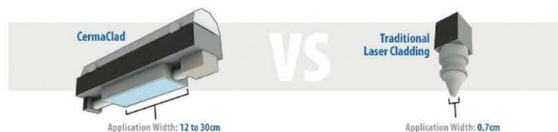
FIGURE 1: CERMACLAD ARC LAMP'S 40 TIMES WIDER APPLICATION AREA COMPARED TO WELD OVERLAY COUPLED WITH RAPID FUSION, LOW HEAT AFFECTED ZONE, MINIMAL DILUTION AND POROSITY ENABLES MESOCOAT TO PRODUCE CLAD PIPES AT RATES UP TO 100 TIMES FASTER THAN WELD OVERLAY.
