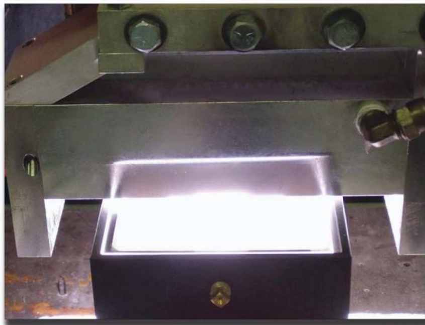
A high-density infrared (HDIR) plasma arc lamp melts a nickel-based alloy material onto a substrate. Photo courtesy of MesoCoat, Inc.
